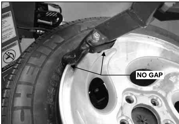
CORRECT (FULLY SEATED) MOUNT/DEMOUNT HEAD
