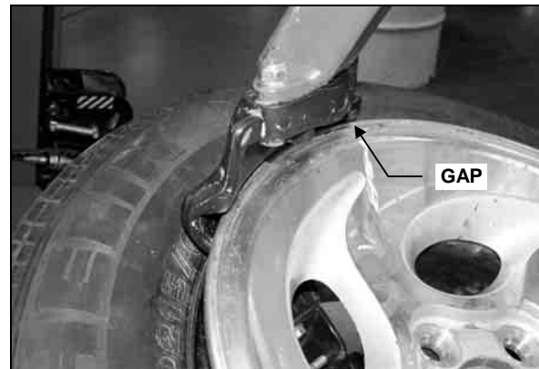
INCORRECT (NOT FULLY SEATED) MOUNT/DEMOUNT HEAD
