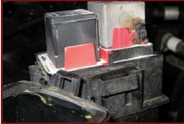
(LEFT) I smelled this before I actually saw it, because the cover hid the damage. My temperature gun measured the relay at a blistering 230 degrees and climbing. The internal short was feeding power from the common circuit on the relay back through the coil, which, in turn, fed back through the EEC circuit to the PCM and all the PCM-controlled solenoids on the same circuit. It was enough voltage to wake up the PCM, but the voltage dropped as soon as the fuel pump ran. This caused the cyclic ticking noise. (RIGHT) Here's the relay without its grey shell. Notice the scorching between the heavy primary terminal and the coil.
