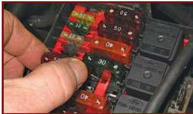
When I pulled this fuse, the clicking stopped. The schematic led me from this fuse to the High Current Fan Relay, which, by this time, I could smell.
